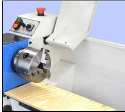
Figure 3-6 Protect the bed when removing or replacing a chuck Chucks, faceplates and wrenches can seriously damage the bed if dropped.
