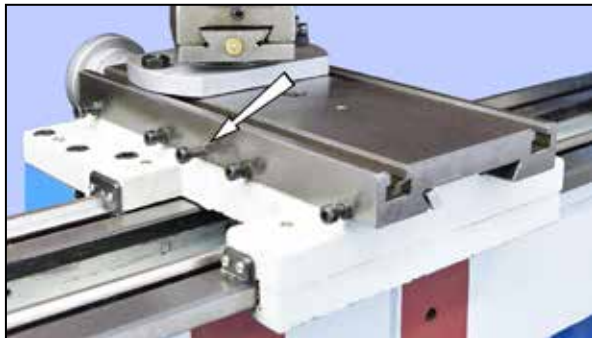
Figure 4-9 Cross-slide gib screws (four) Arrowed screw is the lock screw
