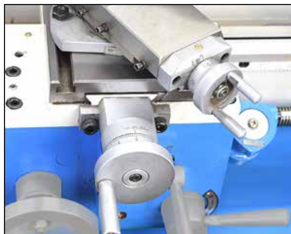
Figure 3-10 Cross-slide and compound dials Both collars are friction-coupled to their leadscrews by leaf springs. To zero a dial, or set it to any desired number, hold the handwheel firmly, then rotate the knurled rim.
