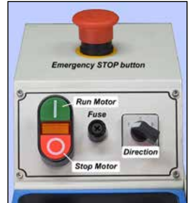
Figure 3-2 Motor controls & tachometer Spindle direction switch: F = Forward (counter-clockwise, as viewed from the tailstock); O = Off, power disconnected; R = Reverse (clockwise, viewed from tailstock). Push buttons: motor ON, GREEN (I) button; motor OFF, RED (O) button.
