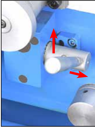
Figure 3-17 Saddle feed Lever RIGHT and UP
