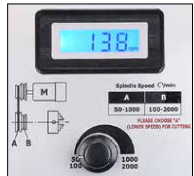
Figure 3-3 Spindle speed control & tachometer
