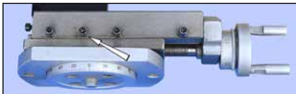
Figure 4-10 Compound gib screws (three) Arrowed screw is the lock screw
