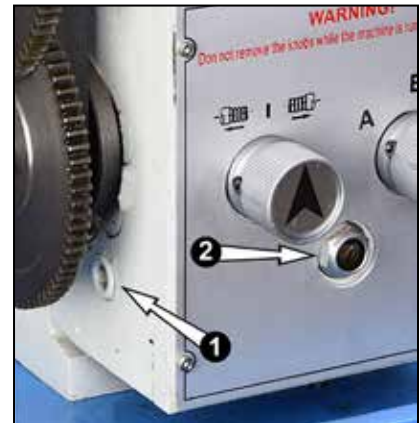
Figure 4-1 Gearbox drain plug (1) & sight glass (2)
