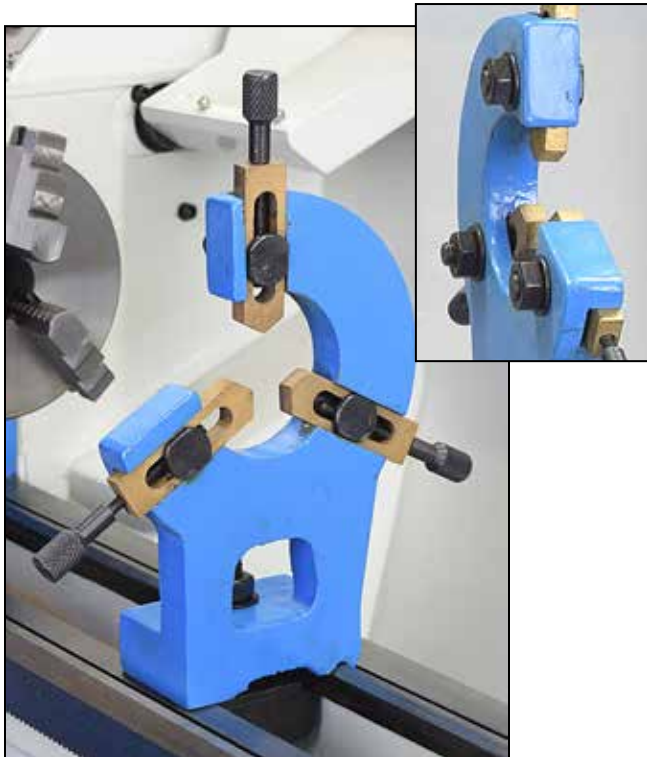
Figure 3-27 Steady rest Maximum diameter 1-1/2 in.
